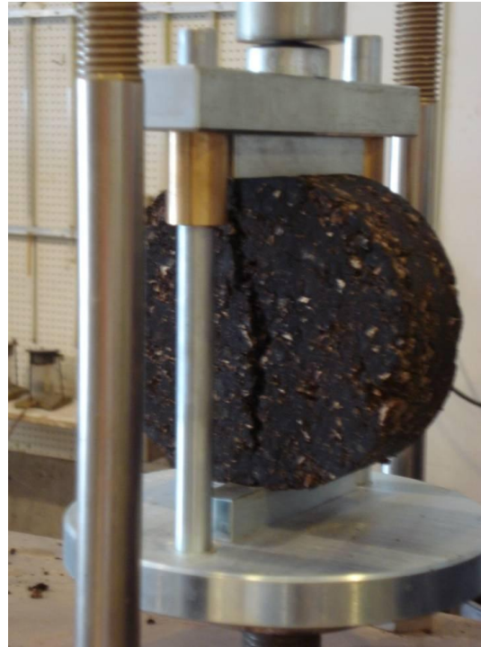
Indirect Tensile Strength (ITS) Testing
