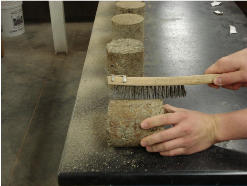
Moisture Sensitivity Testing with Wire Brush Method
